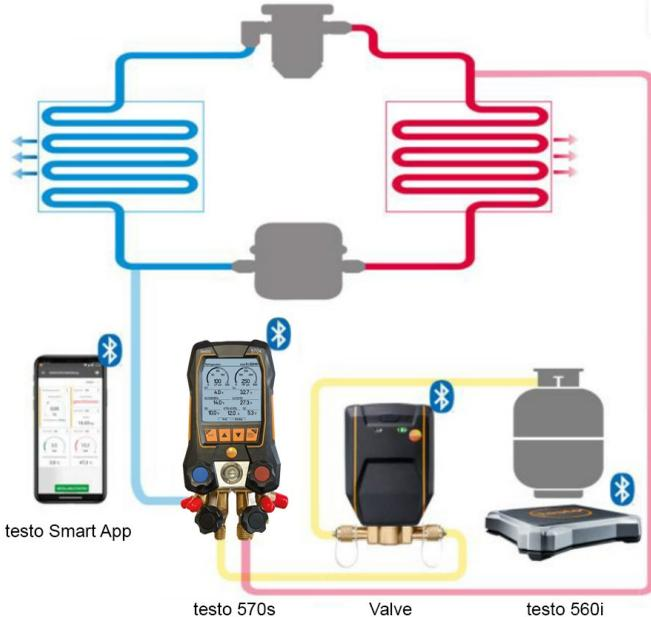
In combination with **testo 560i** and the **testo Smart Valve** the **testo 570s** offers multiple functions to charge refrigerant systems.
