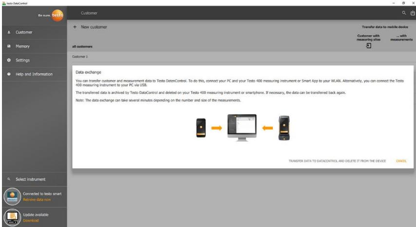
5 Click on **Transfer data to DataControl and delete from instrument.**
