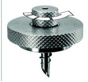
The probe shaft can be guided through the opening of the can and bottle attachment into the can or bottle.
