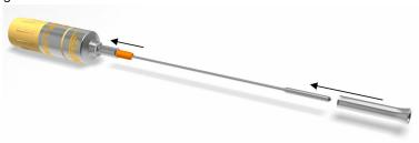
Thread the stainless steel kink protector (2) with straight opening onto the probe and also push it over the plastic clip as far as it will go.
