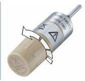
2 Remove battery from the data logger.
